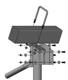
**4 - Diagonal Wind Brace:** Provides increased resistance to wind loads. Primary telescopic section is constructed from  $1\frac{1}{4}$ " Schedule 40 galvanized pipe. Includes 3/8" assembly hardware.
