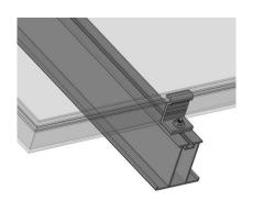
9 - Solar Module Mid Clamp: Fastens two adjoining solar panels in a row to the SF Rail. Mid Clamps are fastened with 18-8 Stainless  $\frac{1}{4}$ -20 T-Head bolts and K-Lock nuts. Clamps are mill finish aluminum.
