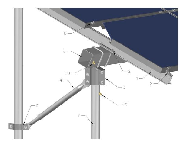
1 - SF Rail: Standard rail lengths are available for 4, 5 & 6 rows of panels in a landscape configuration. Custom lengths are available for a maximum of 8 rows of panels in a landscape configuration or a maximum of 5 rows of panels in a portrait configuration. Rail lengths allow a maximum short side panel dimension of 48" and a maximum long side panel dimension of 96".
