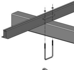
3 - Column Cap: Fastens a horizontal square or rectangular beam to the support column. Includes 1/2" square bend U-bolt sized for specified beam and 3/8" column cap assembly hardware. When required, the Diagonal Wind Brace connects directly to the South column cap. All parts are hot dipped galvanized.
