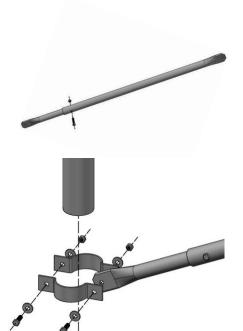
**5 - Wind Brace Column Connector:** Fastens the Diagonal Wind Brace to a vertical column. Includes 2 Column Connector halves and 3/8" assembly hardware. All parts are hot dipped galvanized.
