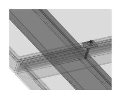
10 - Ground Lug: Installed at any one of the approved locations to provide complete Solar Foundations Ground Mount System grounding. Approved grounding lugs are detailed in the installation instructions.
