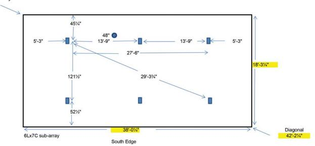
For this 6Lx7C example (6 panels high in landscape by 7 panel columns wide), the 18'-3¼" is the **north-south distance** of the array projected onto the ground. The **east-west dimension** of the array is 38'-0¼".
